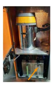
4 Re-fill the water tank (in option without permanent water connection).
