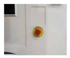
In emergency situations, that can endanger operators health or may result in damage to property, the red emergency button should be pressed immediately. The power will be cut off.
