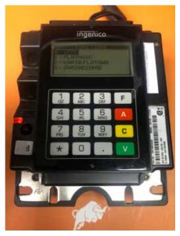
4 Using "F" button go to "SETTINGS" and press "V", as password write 2008 and press "V".
