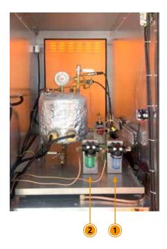
Check the cleanness of the water filter, if dirty should be cleaned.
