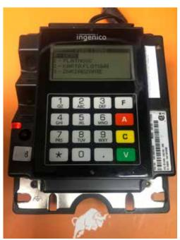
Using "F" button go to "SETTINGS" and press "V", as password write 2008 and press "V".
