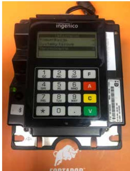
7 Enter TID unique identification number and press "V". Terminal will automatically start configuration process and finally make re-start.
