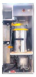
4 Re-fill the water tank (in option without permanent water connection).
