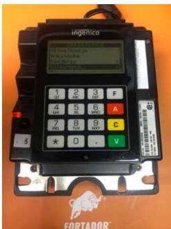
5 Using "F" button go to "SERVICE" and press "V"
