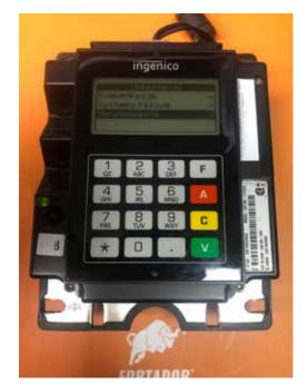
7 Enter TID unique identification number and press "V". Terminal will automatically start configuration process and finally make re-start.
