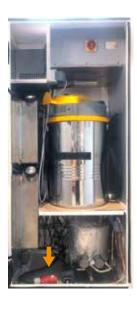
2 Check the cleanness of the water filter, if dirty should be cleaned.
